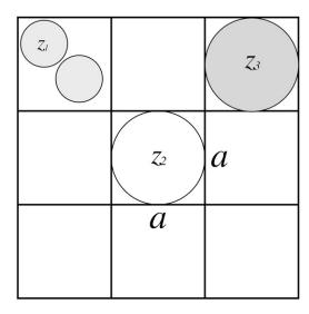
FIGURE 1 Schematic illustration of the lattice gas model. The lattice size a sets the size of the species with valences  $z_2$  and  $z_3$  while the k parameter (in this case, k = 2) sets the relative size of the smaller ion with valence  $z_1$ .
