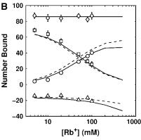
FIGURE 5 SMPB (solid) and PB (dashed) prediction for CC =  $\text{Li}^+$  (A) or Rb<sup>+</sup> (B) competing against BC = 50 mM Na<sup>+</sup> around a 44-bp DNA duplex. Net charge ( $\diamondsuit$ ), CC ( $\square$ ), fixed BC ( $\bigcirc$ ), and co-ion ( $\triangle$ ). SMPB curves were computed using size parameters obtained from fitting against 50 mM Na<sup>+</sup> 24-bp duplex competition data.
